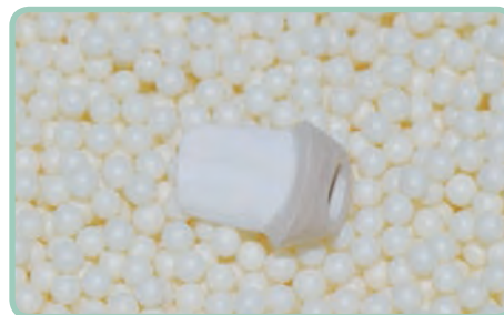
A sintering process is required when zirconia is used
